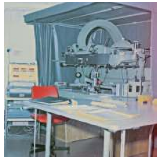
A Wild B8S with tri-axis locator and EK8 which provided a digital read out of co-ordinates thus providing an aerial triangulation capability.
