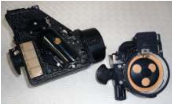
The clockwork 'mean' averager of the RAF MkIXA compared to the score-mark 'median' averager of the USAAC Mk10a sextants (DP).
