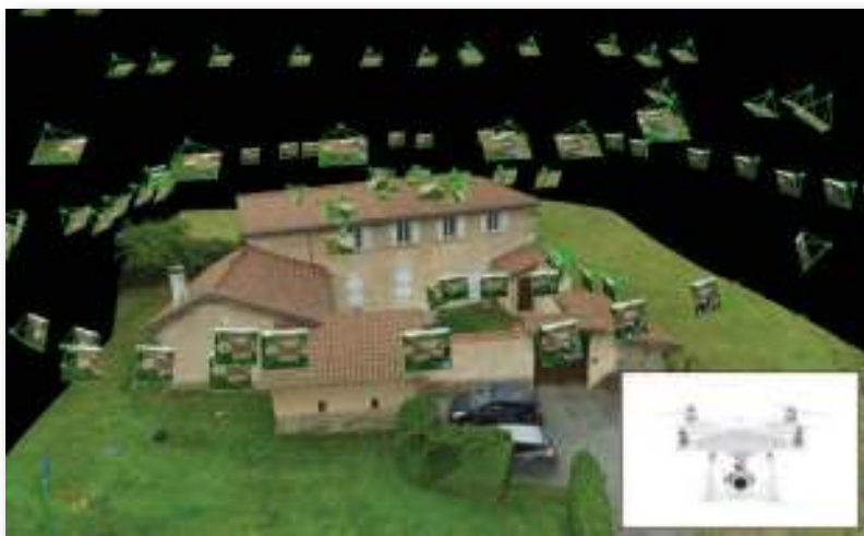
A snapshot of a 3D model, created from multiple stills taken by a small COTS UAV currently being trialled by 42 Engr Regt (Geo) (image courtesy of Pix4d).
