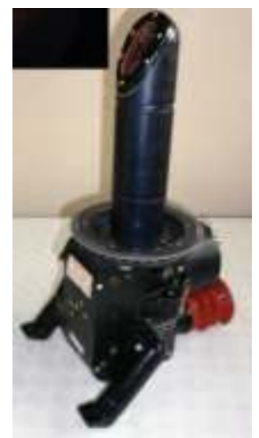
An RAF Smiths Mk2b Pendulous Reference Periscopic Sextant with the view to the Observer inset (DP).
