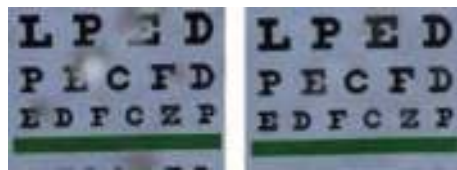
Figure 4 – Image portion under rain conditions (on the left) in direct comparison to after lucky imaging processed image (on the right). Due to camera speed restrictions, only five images were acquired and processed. From: Marsh, 2016.
