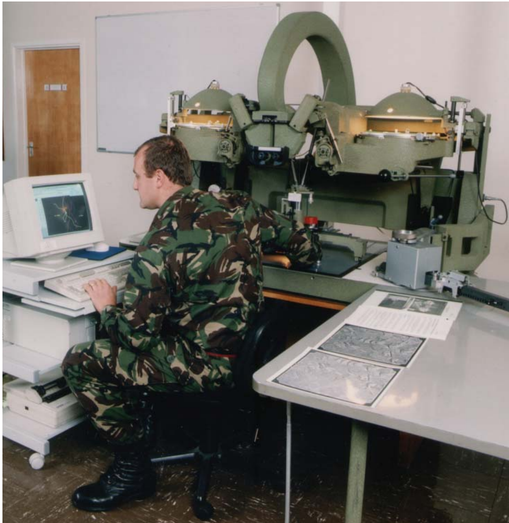
Fig 1: Wild B8 with DAT-EM, a customised version of MicroStation attached
