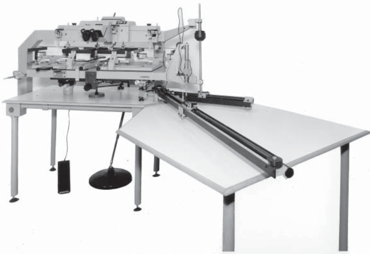
Professor Thompson's CP1 Plotter: one of these instruments has been preserved in the Science Museum store at Wroughton
