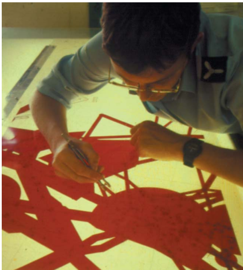
A positive mask being produced using Cut and Strip techniques
